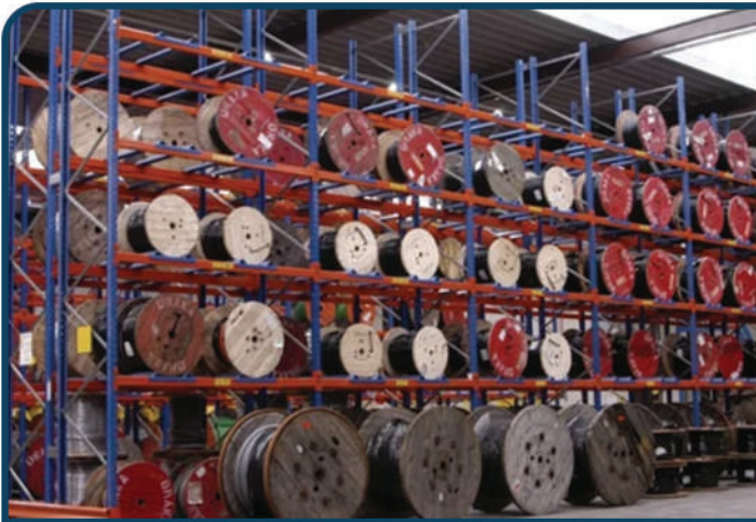
Cable Drum Storage Rack
